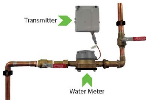
A small box, called a Meter Interface Unit (MIU), or transmitter, is installed on the interior of your house or business near your water meter. It is connected to your new water meter inside your home, and transmits a radio signal to a data collector, which is then transmitted to the City. Each meter has a unique identification number that ensures only your reading is assigned to your account. This system reduces the need for meter readers to manually gather meter readings.
